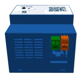
Dimensions: 4 DIN modules (length: 95 mm, width: 71 mm and height: 58 mm)
